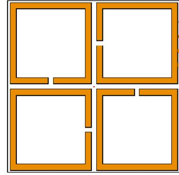
Figure 8. Arrangement of loaded loop for realization of dual-polarized AMC surface (dimensions is similar to that in Fig. 4).
