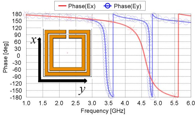
Figure 7. The reflection phase of dual-band unit cell when the position of both gaps is the same.
