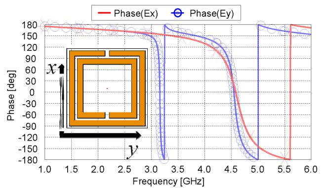
Figure 9. The reflection phase of dual-band unit cell when the position of gaps is different.
