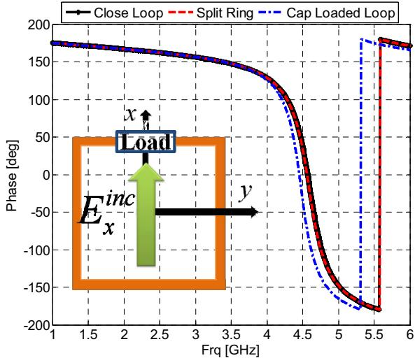
Figure 3. The reflection phase of different loaded loop (in Fig. 4) for  $E_x$  as a incident electric field polarization.
