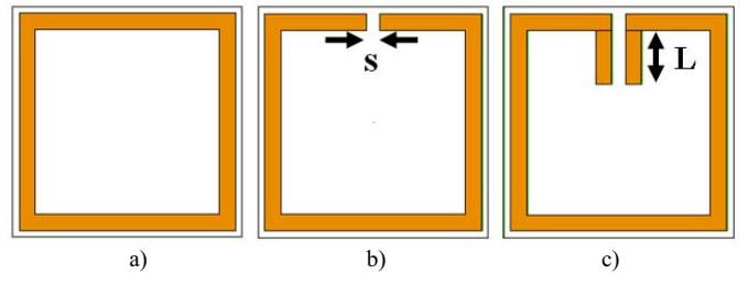
Figure 4. The unit cell of different loops,  $s=0.3$  mm,  $L=1.17$  mm, (Fig. 1. parameters:  $d=5$  mm,  $\alpha=4$  mm,  $w=0.35$  mm).
