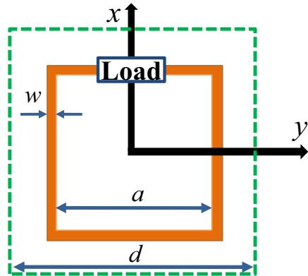
Figure 1. Loaded loop unit cell.
