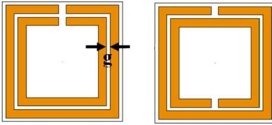
Figure 6. Multiband unit cells based on the use of loaded loop with different resonance lengths.  $g=0.15$  mm (both ring have same “ $w$ ” and dimensions is similar to that in Fig. 4)
