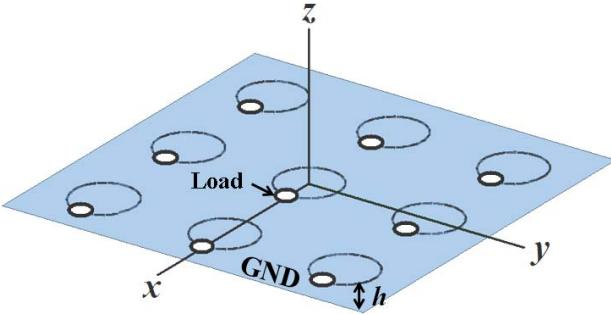
Figure 2. Planar regular array of loaded loop over a grounded dielectric slab ( $h=1.6$  mm and  $\epsilon_r=10.2$ ).
