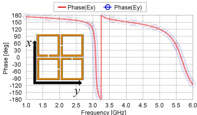
Figure 10. The reflection phase of dual-polarized arrangement (Fig. 8) of split loop for  $E_x$  and  $E_y$  polarization.
