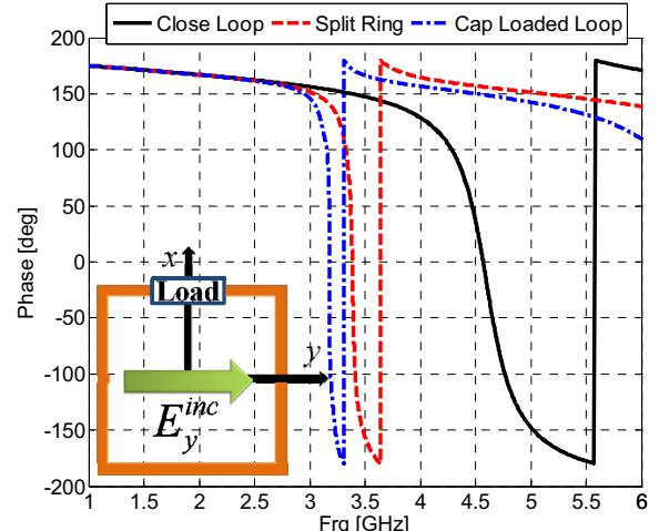
Figure 5. The reflection phase of different loaded loop (in Fig. 4) for  $E_y$  as a incident electric field polarization.
