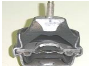
Fig24. Hydraulic engine mount with Inertia track
