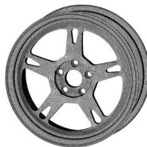
Figure 23: Re-meshed model of wheel
