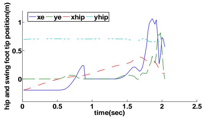
Fig. 4 Vertical and horizontal tip position of hip and swing foot in the fixed foot length mode
