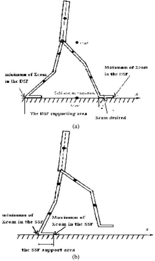
Fig. 2 (a) The DSP and (b) the SSP supporting area and their margins
