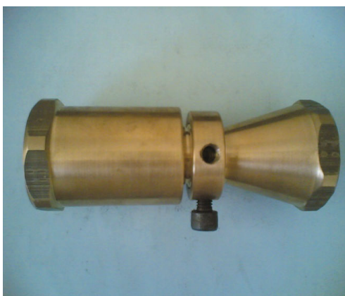
Fig. 13. Schematic of optimum venturi
