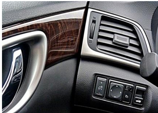
Fig7. Applying texture on interior components decreases glossiness, which leads to a vivid vision when looking at the buttons
