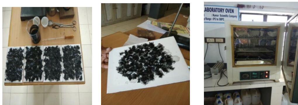
Fig 2.5 Grafting MWCNT-F on CF Surface
