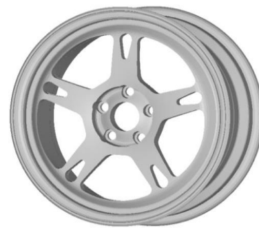
Figure 20: The optimized design after topology optimization
