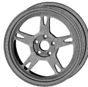
Figure 23: Re-meshed model of wheel
