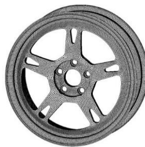
Figure 23: Re-meshed model of wheel
