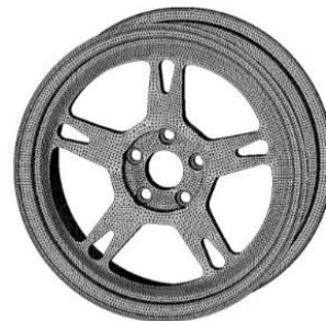
Figure 23: Re-meshed model of wheel
