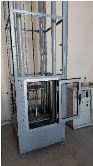
Figure 8: DCB impact test setup.
