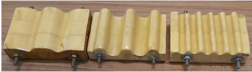
Figure 20: Corrugated wooden molds
