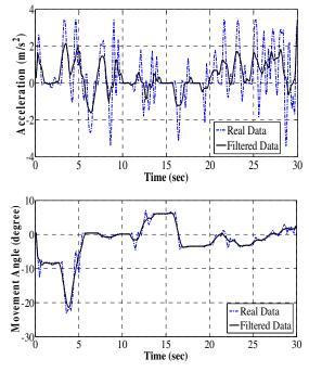
$\textbf{Fig6.} Comparison \ of \ unfiltered \ and \ filtered \ data: (a) \ Longitudinal \ acceleration, (b) \ Movement \ Angle.$
