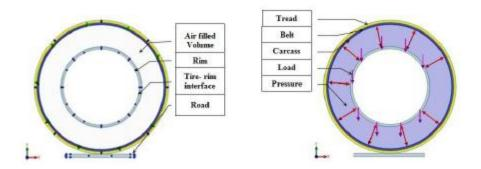
Fig4. Imposing of boundary conditions for radial tire.
