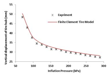
Fig5. Tire hub displacement versus inflation pressure.
