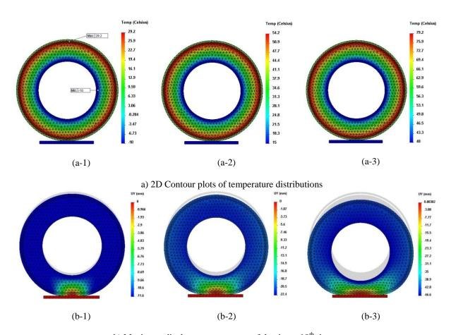
b) Maximum displacement contours of the tire at  $10^{th}$  time step Fig8. Temperature and displacement distribution on the tire for three different ambient temperatures, a) -10 °C; b) 15 °C; c) 40 °C.
