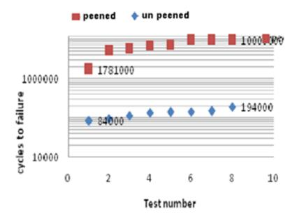
Fig13. Experimental fatigue life testing results of connecting rods, manufactured from (Fe Cu C) powder [9].
