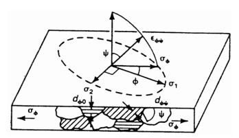
Fig1. Plane stress in a free surface [12].
