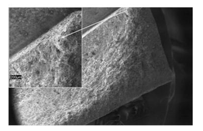
$\textbf{Fig9.} \textbf{SEM} \ \text{micrograph} \ \text{of fractured surface} \ \text{of unopened part, fatigue crack started from surface}.$
