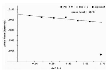
Fig7. Distance of stressed planes(d), versus Sin2ψ, third row of Table(3).
