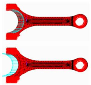
Fig5. Compressive (-17,810N) and Tensional (7,870N) Loading.
