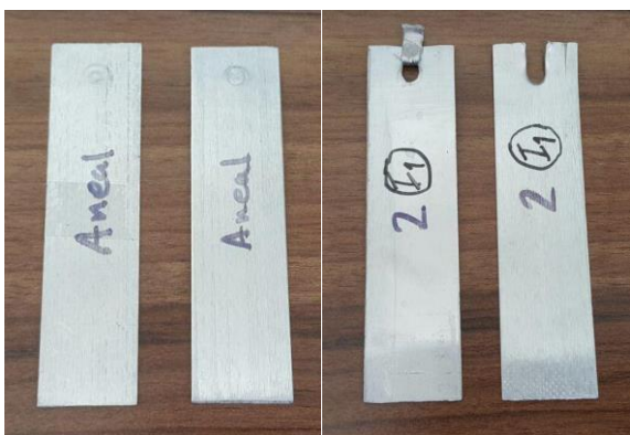
Figure 4: Failure modes. Left: IF failure mode - Right: PF failure mode
