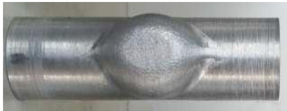
Figure 13: deformed tube (sample T.5, thickness of 2.1 mm) [15]
