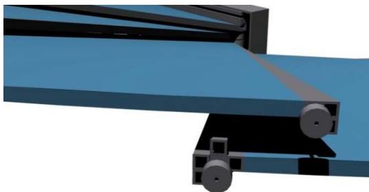
Fig. 19. A view of two adjacent parts of a retractable section
