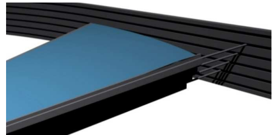
Fig. 20. Telescopic bars attached to triangular parts for making a connection to linear tracks
