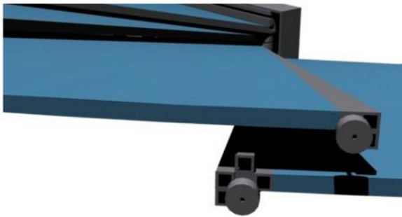
Fig.20 Section of panels' profile in adjacent panels.
