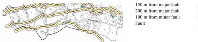
Figure 6: Border of the fault
