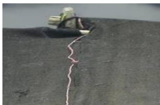
Fig 34. Method of connection of the two strips of fabric by metal pins
