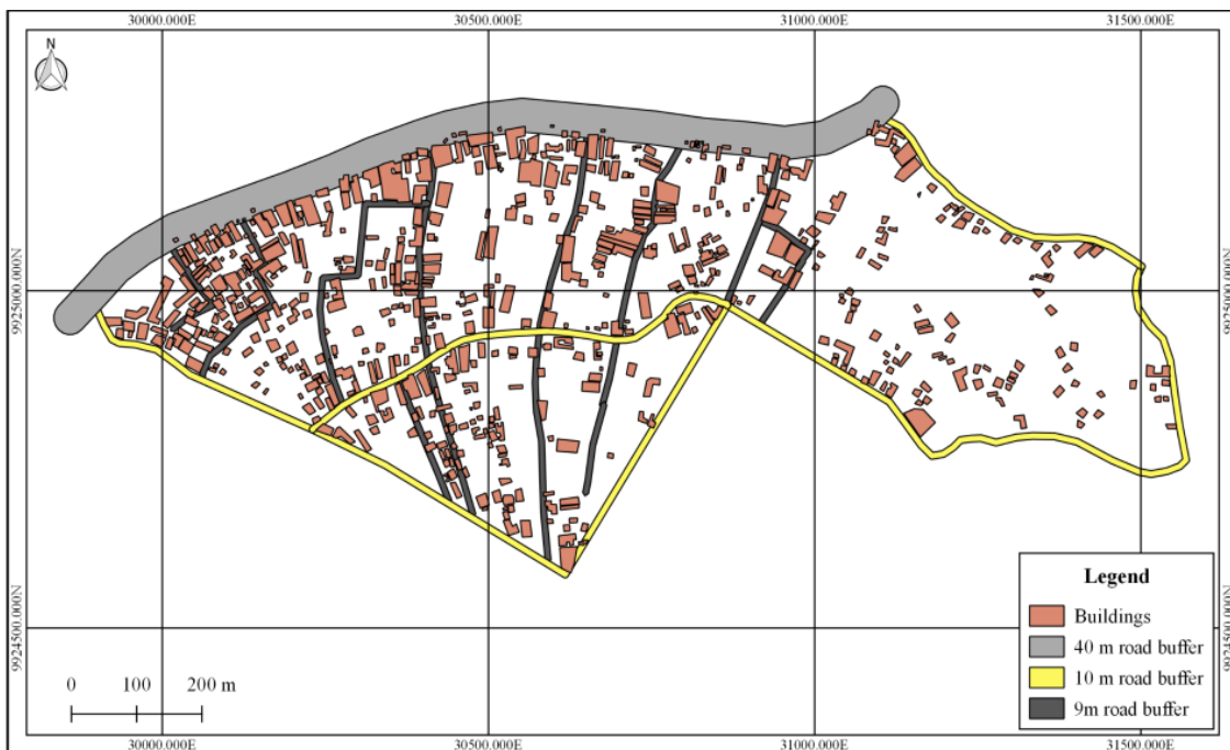
Fig 5. Encroachment of planned road reserves in a selected section in Jogoo
