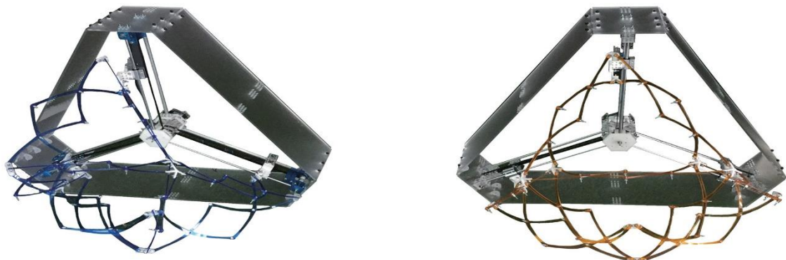
Fig 10. The Adaptive Component Triggered Closed and Open States through Motion (Chang et al., 2019)
