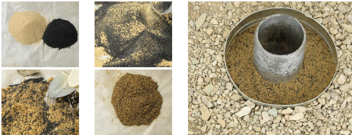
Fig. 10 Preparing the Soil-Rubber Mixture and Constructing Iso_M Model
