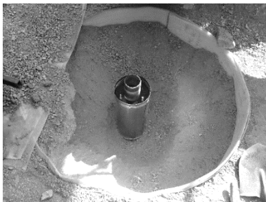
a. Excavation of 0.6 m of top of the Con model
