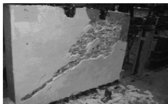
Fig 13 Separation of plaster due to crack formation in specimen B at last loading step
