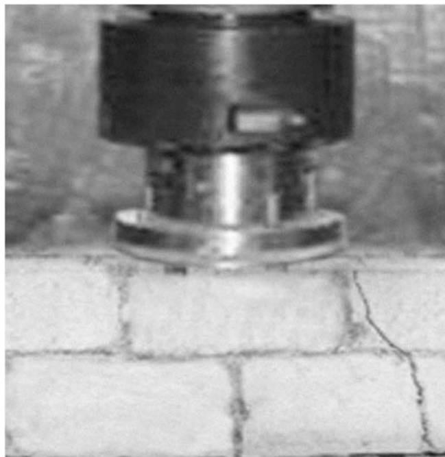
Fig. 3 Shear Failure for Beam Tests
