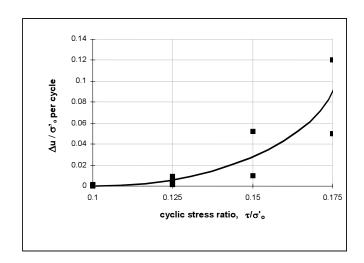
Figure 1. Pore water pressure ratio increase per cycle during steady state phase for medium dense carbonate sand.
