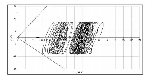
Figure3. Effective stress path for loose carbonate sand under a cyclic stress ratio of
