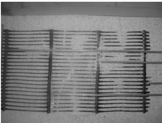
Fig. 4. Sample preparation and installation of nodal displacement measurement system
