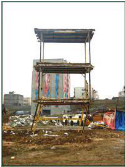
Fig. 4. Pullback test of the safe room located at the ground-floor level
