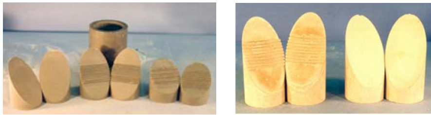
Fig. 2. a) The molds for casting the specimens, b) Prepared smooth and rough surfaces
