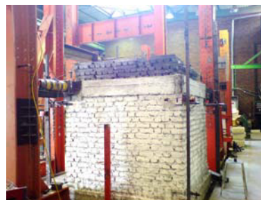
d) Instrumented specimen ready for test
