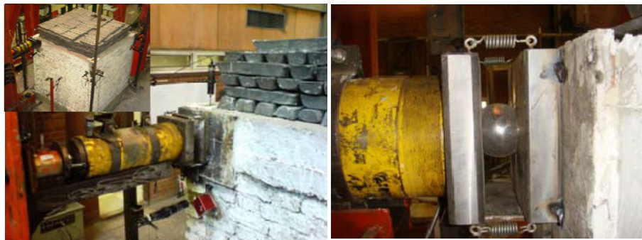
b) Application of loading system
