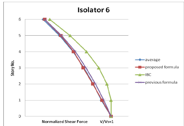
Fig. 14 Comparison of nonlinear dynamic analysis, IBC formula, proposed formula in section 6 and previous formula for 6 story building
