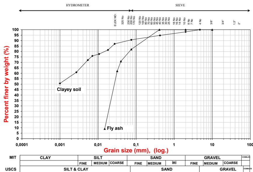
Fig. 3 Grain size distribution curves of fly ash, clayey on the base of sieve and hydrometer analysis.
