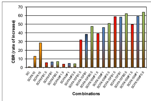
**Fig. 11** Different fly ash, fibrillated polypropylene fibers (F19average) and multifilament fibers (MF19average) content increase in CBR values
