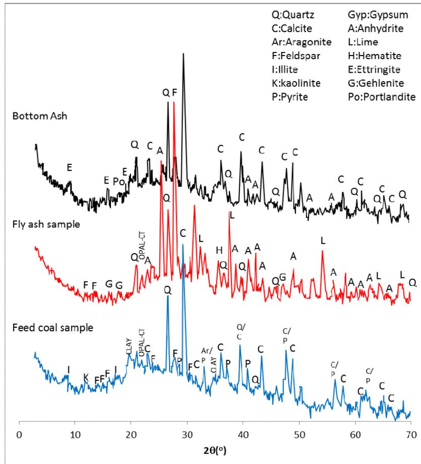
**Fig. 4** Selected examples of X-ray diffraction traces of feed coal , fly ash and bottom ash from the Kangal power plant, Turkey.
