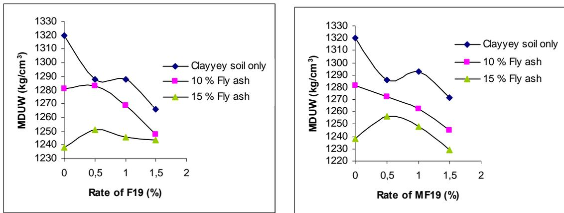
**Fig. 7** The variation of maximum dry unit weight
