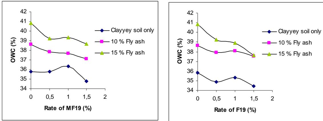
Fig. 8 The variation of optimum water content
