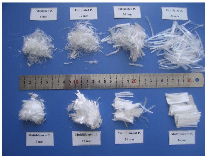
Fig. 6 Multifilament fibers and fibrillated polypropylene fibers used in this study (as supplied by the manufacturer)
