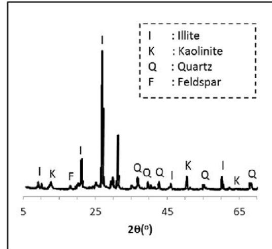
Fig. 2 Characteristic XRD graph of clayey soil used.
