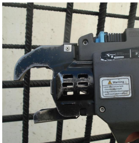
Fig. 4 Close-up of the adjustable pick
