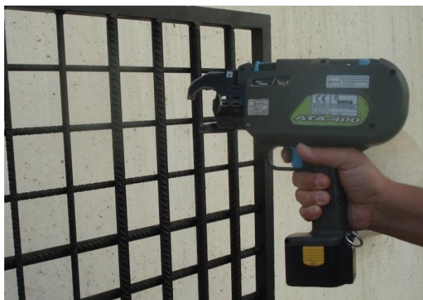
Fig. 6 Battery powered rebar tier
