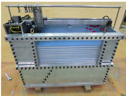
Fig. 1 Fault simulation container
