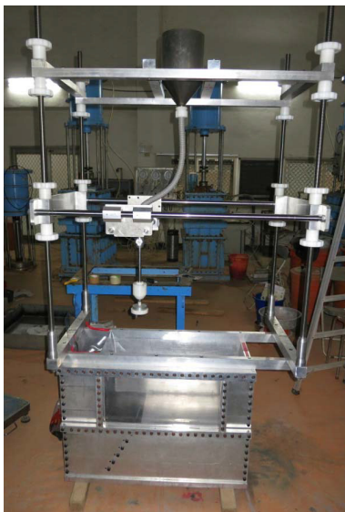
Fig. 5 Sand pluviator on the fault simulation container
