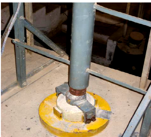
Fig. 1 Disc specimen under drop weight impact test
