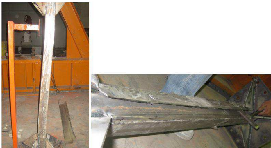
Fig. 27 Core buckling under the second mode
