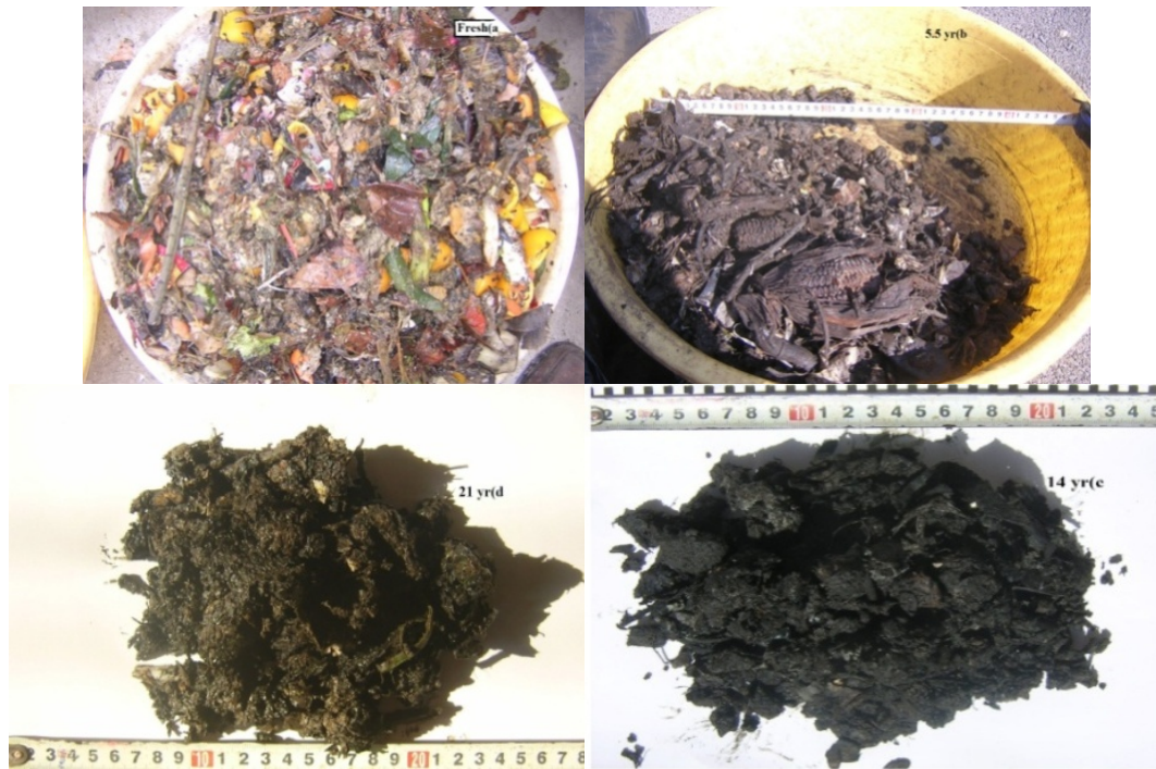
Fig. 5 Visual status of paste contribution for different samples: (a) fresh waste, (b) 5.5-year-old sample, (c) 14- year-old sample, (d) 21-year-old sample
