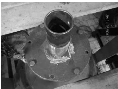
Fig.10. Details of steel model piles driven in FCV with Casing guide
