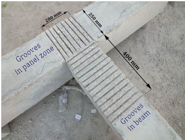
Fig. 2 Grooving pattern in specimen RW2
