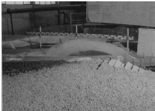
Flip Bucket Model of Jareh Dam
