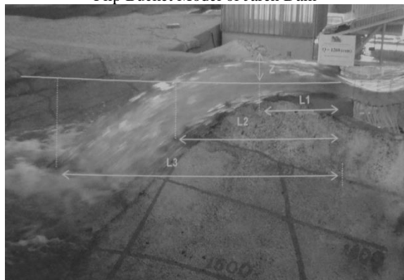
Flip Bucket Model of Ajab Shir Dam
