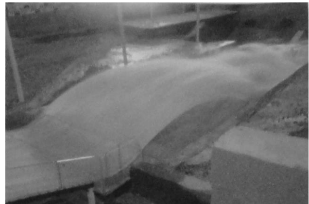
Flip Bucket Model of Azad Dam
