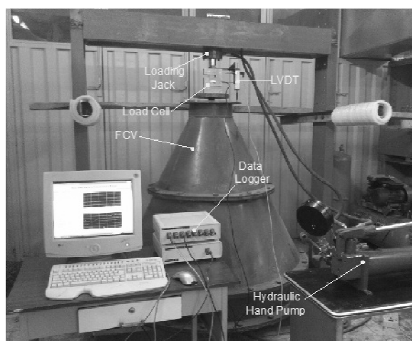
Fig. 4 Overview of FCV at AUT and its accessories
