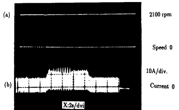
Fig. 5 Speed and dc link current responses to step load at 40 Hz. (a) conventional control speed at 1200 rpm [6] (b) conventional control dc current [6] (c) proposed control speed (d) proposed control dc current.
