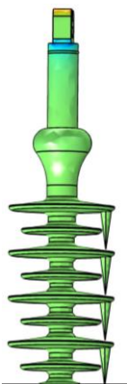
Fig. 9 Modeled icicles on the insulator shed.
