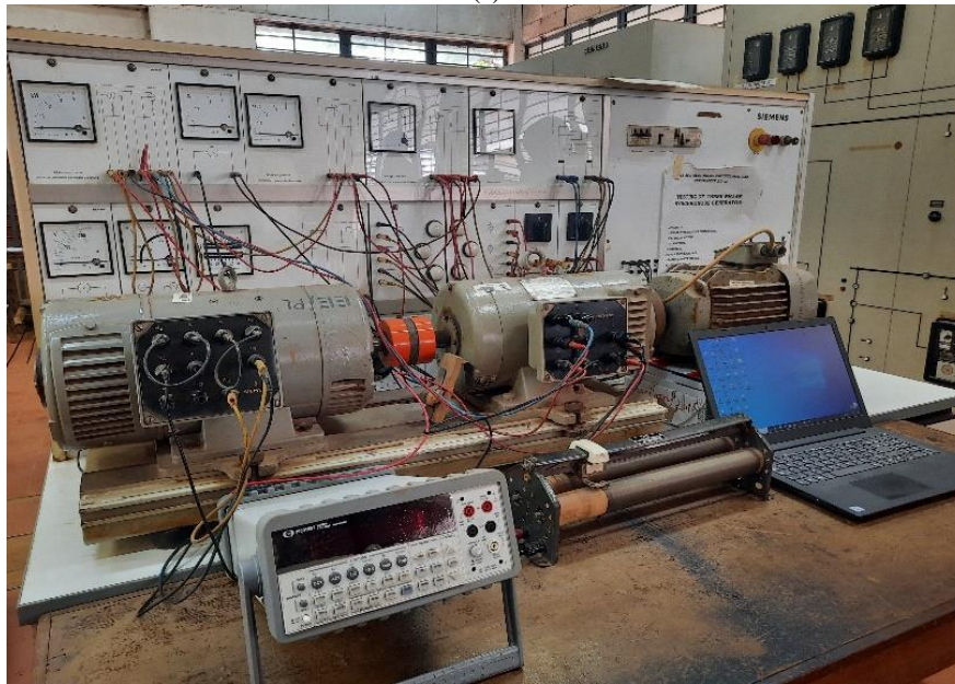
Fig. 10 The experimental setup of the hybrid machine; a) Connection diagram and b) Photograph.
