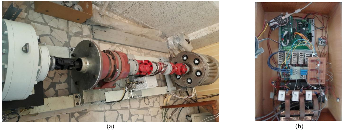
Fig. 5 Test setup; a) the fabricated BLDC permanent magnet motor during testing on a dynamometer and b) the fabricated drive.
