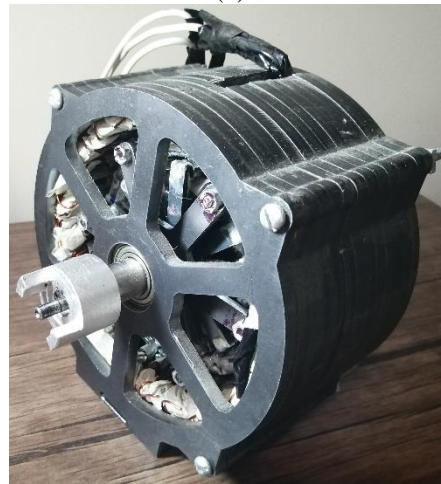
Fig. 8 The MCMG machine, (a) internal rotor and modulator, (b) external rotor (c) the final machine.
