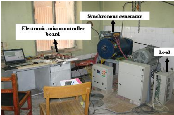
Fig. 4 Testing laboratory and experimental test setup.
