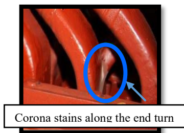
Fig. 6 Corona at interface at the first crossover [19]
