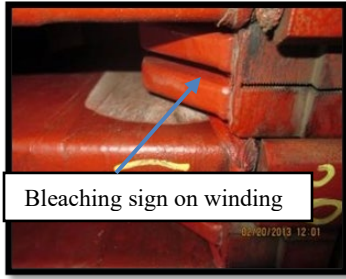
Fig. 4 Bleaching sign on windings [19]
