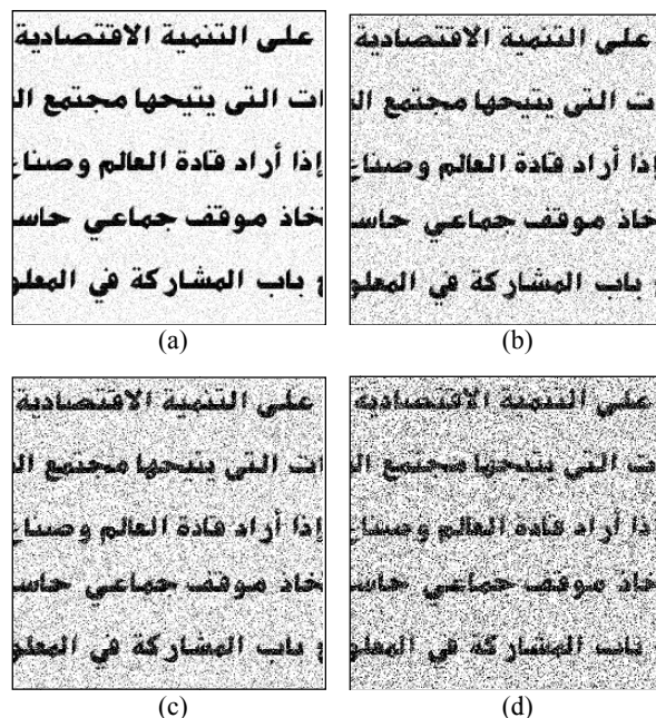
Fig.16 Example of noising images with various values of SNR: (a) SNR=50, (b) SNR=40, (c) SNR=30, (d) SNR=20.
