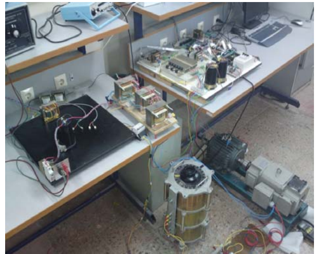
Fig. 4 SRM drive test setup used for experimentation.
